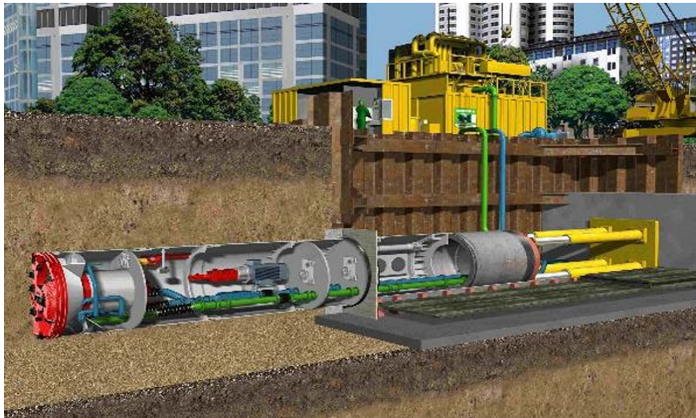
Plate 3.10: Indicative micro-tunnelling schematic
